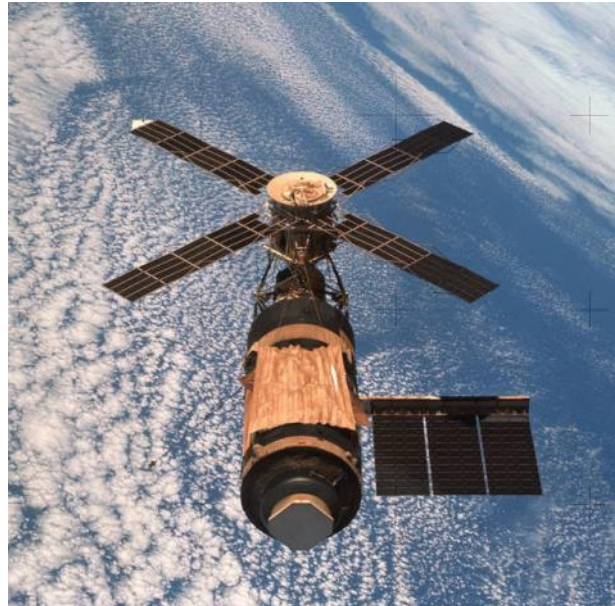
Skylab photographed by the final mission crew as they left on 8 February 1974. The sunshield is over the section nearest the camera. The lost solar panel wing should have been on the left side.
